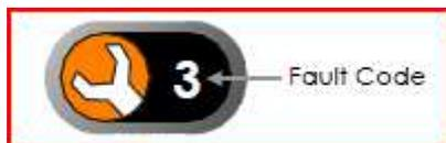
In the case of a fault; the DX2 controller may display a flash code like the one pictured. The number indicates where the problem is in the system. The following information may help diagnose some faults
