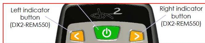
The indicators can be activated with the indicator buttons on the controller. Alternatively, press the accessory mode selection button until the screen shows
