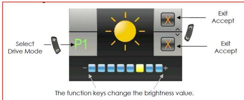
Using either the function buttons or the joystick left/right to change the screen brightness
