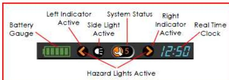
The battery gauge indicates how much charge remains.
