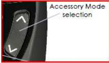
If you are in Drive Mode, a press of the accessory mode selection button will take you to the last used accessory function, e.g. actuator control. If you are already in Accessory Mode, a press of the accessory mode selection will take you to the next available accessory mode, e.g. lighting. To return to Driving, simply press the drive profile selection button.
