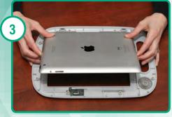
Place the iPad, screen down, into the front piece of the GoNow Case. Align the iPad charging dock with the Case access port.
