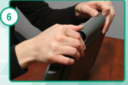
Push out on the top groove of the CoverStand to remove it from the Case.
