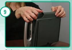
Push out on the top groove of the CoverStand to remove it.
