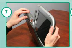
**COVER** Place the GoNow Case into the bottom groove of the CoverStand with the iPad screen facing the inside.
