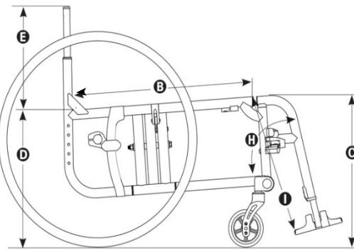
**FRONT SEAT HEIGHT** C Measure from floor to top of seat tube at front edge of seat sling. Adjustable in 1/2" increments. (13.5" - 14" Front Seat Height C requires Hemi Height Frame Style. 20.5" - 21.5" Front Seat Height C not available with Hemi Height Frame Style.).
