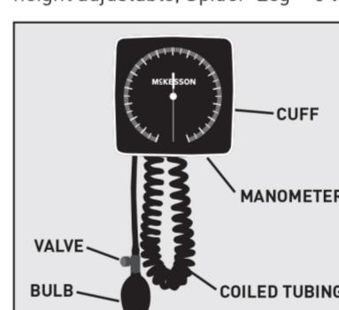
To assemble the inflation system, connect coiled tubing to air inlet nipple at bottom of gauge. Insert male luer adapter on bladder tubing into female receptacle at free end of coiled tubing. Store folded inflation system in swivel bracket behind gauge on 01-750W-11ABKGM or in integral basket on 01-752M-11ABKGM.
