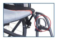
ADJUSTING LENGTH OF FOOTREST/LEG REST - When adjusting length of foot rests or leg rests, user should be sitting in wheelchair with feet on the foot plates. Loosen bolt on the footplate assembly below the heel loops. Raise or lower foot plate to desired position that will provide maximum support of thighs. Front rigging should not be so low that it causes uncomfortable pressure to thighs at front of seat upholstery. Footrest should not be lower than 2-1/2" from the ground to ensure clearance.
